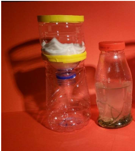
Step 5: Collect some river water & start the filtration process!
